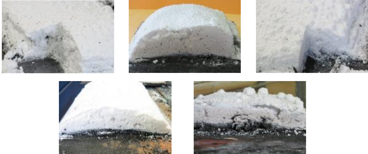
Char structure, after fire testing, of intumescent formulation based on new binder HYDRO PLIOLITE 211, compared to commercial waterborne and solvent-borne intumescent coatings
