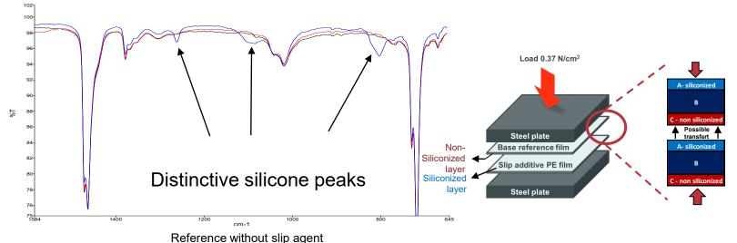
6wt% DOW CORNING<sup>™</sup> MB25-235 Masterbatch non siliconized skin layer after 2 months under weight 6wt% DOW CORNING<sup>™</sup> MB25-235 Masterbatch siliconized skin layer
