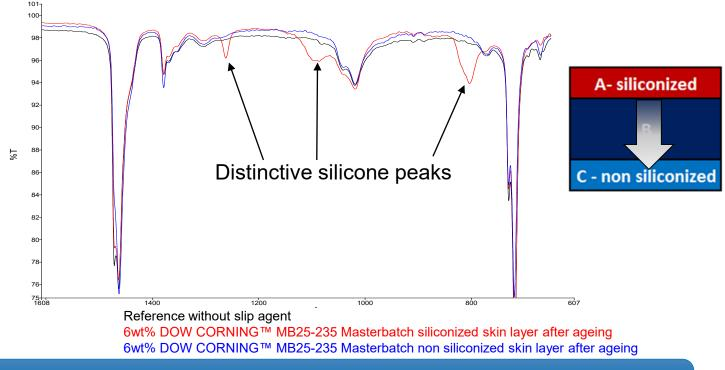
The silicone does not migrate through layers, even after ageing at 60°C for 1 month and even at high loadings.
