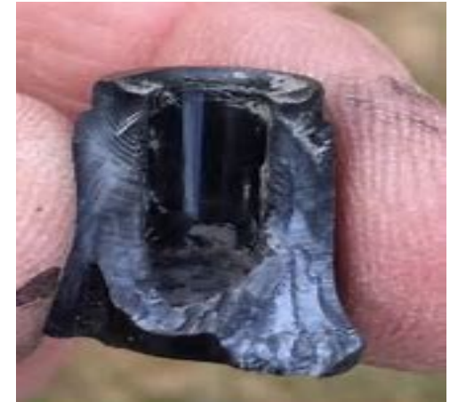
Example of stress cracking fracture on plastic boss
