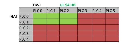
Flame ratings can shrink or enlarge your material options for a given application – i.e. higher flame rating will allow for lower performance against electrical line sources.
