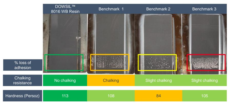
Samples were cured at 200°C for 1 h then exposed to high temperature (500°C, 2 h, on hot plate).
