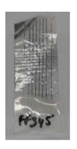
Samples were cured at 200°C for 1 h then exposed to high temperature (500°C, 2 h, on hot plate).
