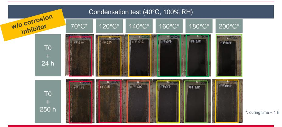
Curing recommendation = 180-200°C (1 h) to ensure sufficient resistance to water
