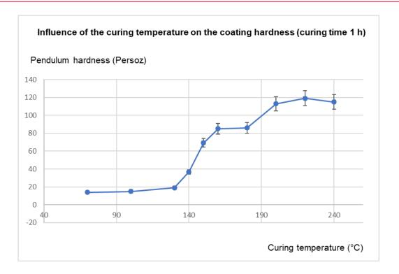
Curing recommendation = 200°C (1 h) or above to ensure maximum coating hardness
