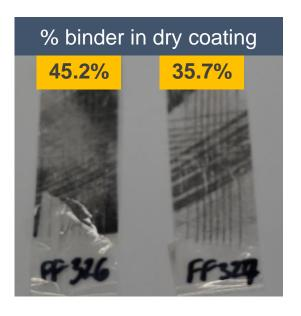
Samples were cured at 200°C for 1 h then exposed to high temperature (500°C, 2 h, on hot plate).
