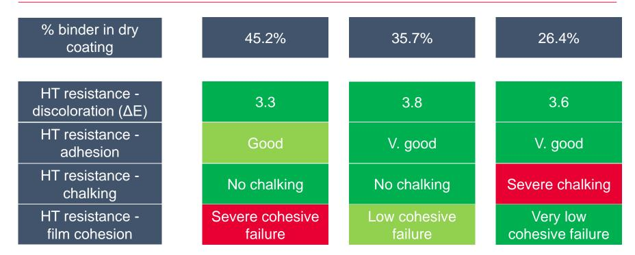
Samples were cured at 200°C for 1 h then exposed to high temperature (500°C, 2 h, on hot plate).
