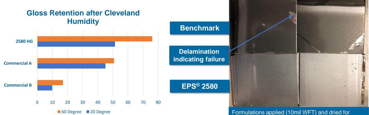
Formulations applied (10mil WFT) and dried for 24hrs. Films were then placed in 60°C Oven for 30min with 1kg weight applied. After 30min, specimens were removed from oven and left at room temp. for 30min with weight still applied. After this the films were separated and assessed for blocking.
