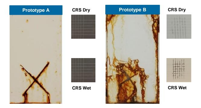
Corrosion resistance tends to degrade as wet adhesion is improved in waterborne acrylic emulsion coatings
