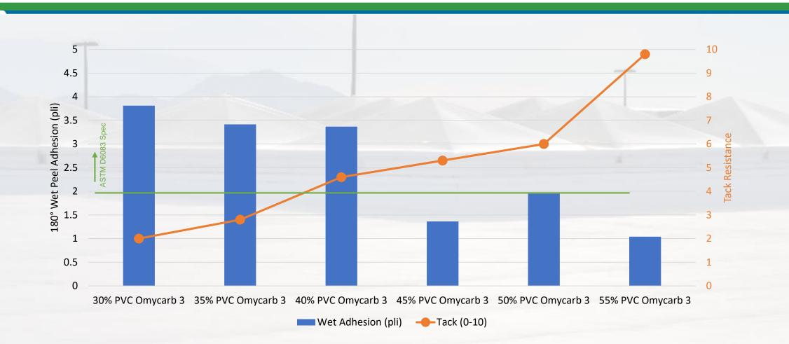
Highly filled systems may negatively impact adhesion and should be evaluated 40% PVC is recommended for an optimal combination of adhesion and low tack
