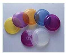
Figure 3 Photochromic polymers (courtesy Colourchange, a division of LCR Hallcrest)
