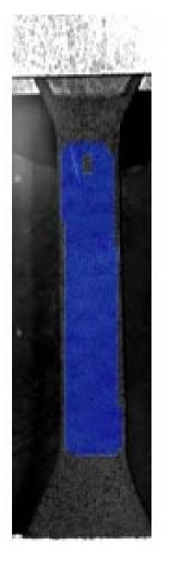
Use of high speed camera and digital image correlation to post process true strain rate
