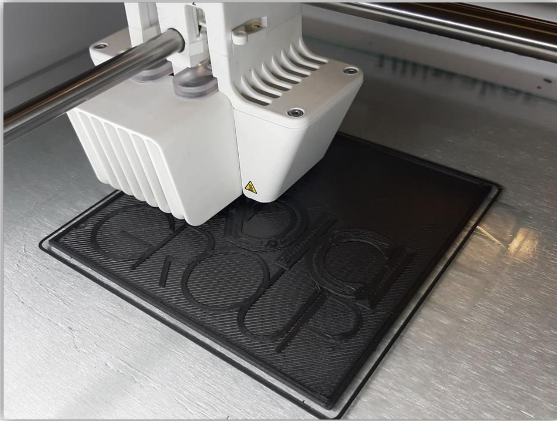
Radilon® Adline printed with Ultimaker S5
