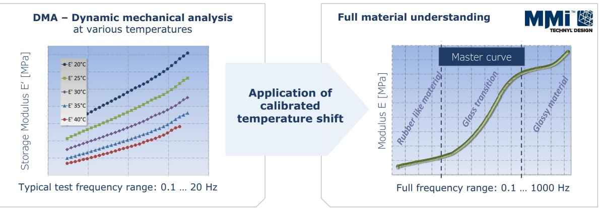
Material master curves are built as basis of anisotropic visco-elastic models considering GF orientations and included in MMI
