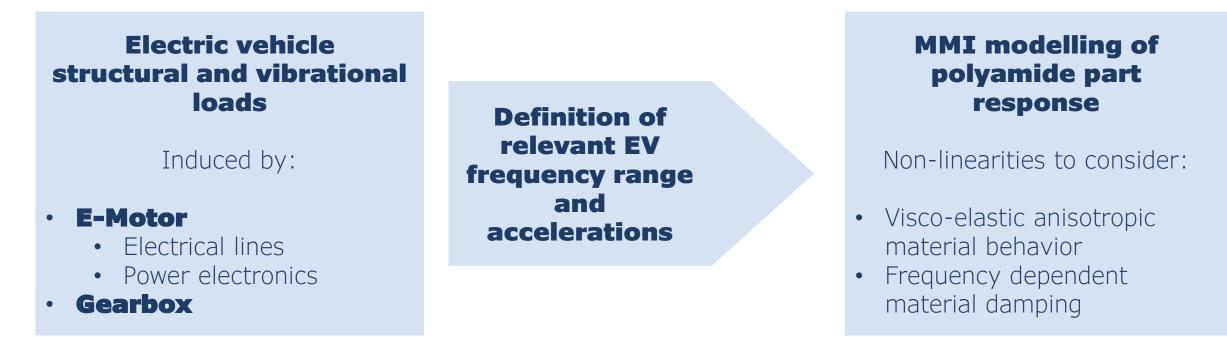
Unlike combustion engines, the e-powertrain emits high frequency and low amplitudes harmonic noise Correctly modelled polyamide components are the basis of system modelling
