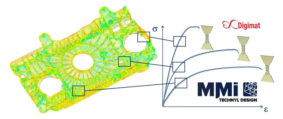
GF orientation specific material properties including damping for each element provided to the FE-Solver
