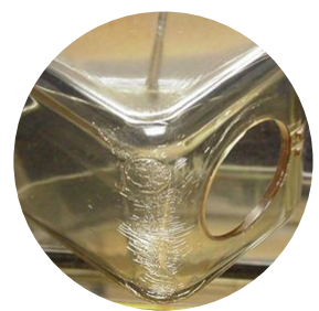
Residual Stress Cracks on Molded Part
