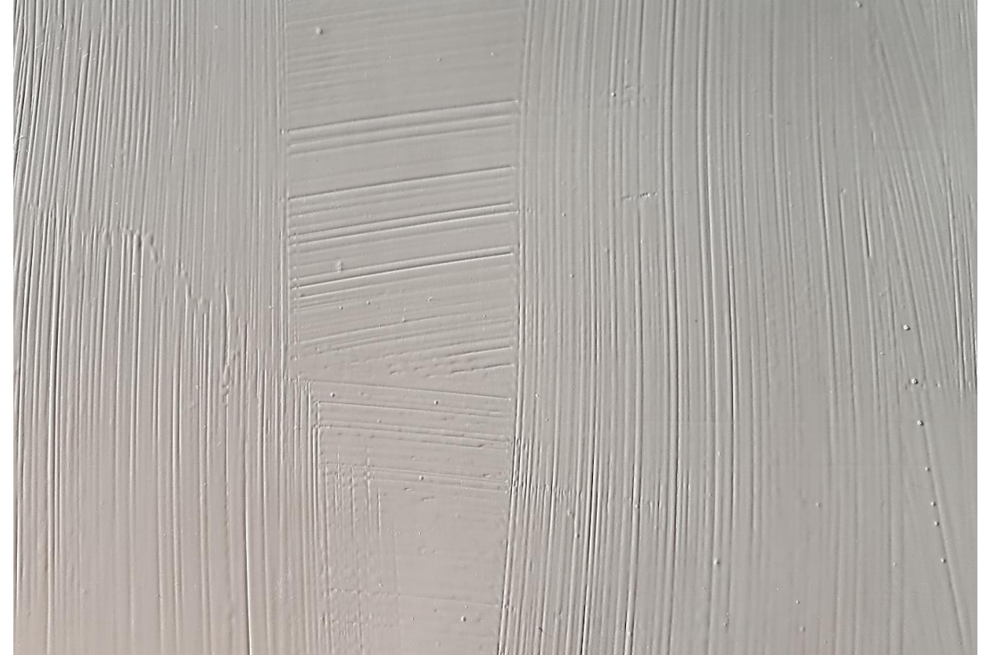
Bad leveling, brush marks due to high viscosity
