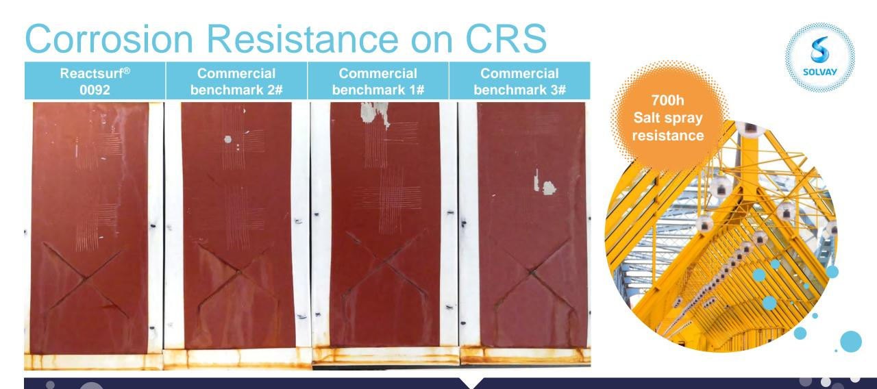
After 700hrs, Emulsion with Reactsurf<sup>®</sup> 0092 still shows satisfactory corrosion resistance. Also the wet adhesion to CRS is much better than all 3 benchmarks with no peel off.
