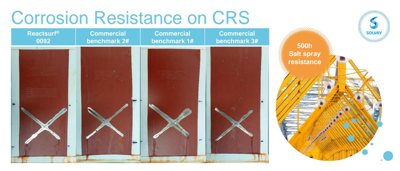
According to the peel off area, Emulsion with Reactsurf<sup>®</sup> 0092 clearly shows better corrosion resistance compared to all benchmarks from the market.
