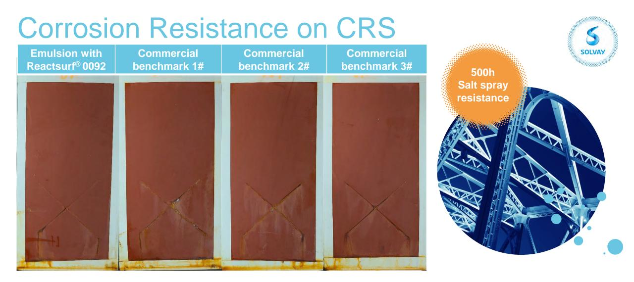
After 500 hrs salt spray test, Emulsion with Reactsurf<sup>®</sup> 0092 shows excellent corrosion resistance.
