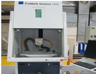
TRUMPF LASER TM 3020 Frequency : 1-100 kHz
