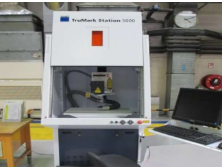
TRUMPF LASER TM 6330 Frequency : 1-120 kHz
