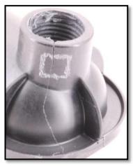
Molding configuration + crack localization
