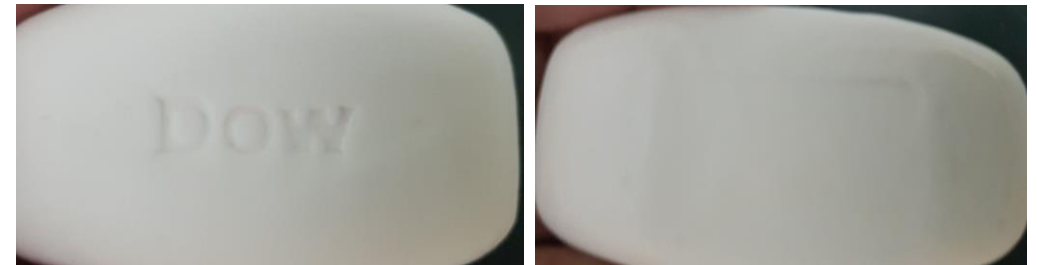
no visual cracking, smooth bars
