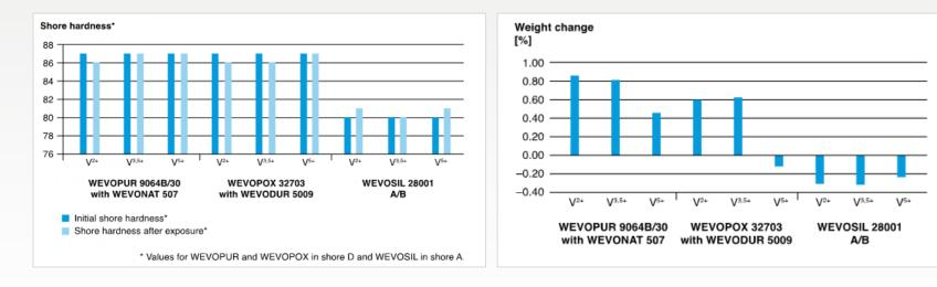
The observed change in Shore hardness was minor for all tested polymers and from this point of view it can be stated that the materials are resistant in the electrolytes at different oxidation levels.
