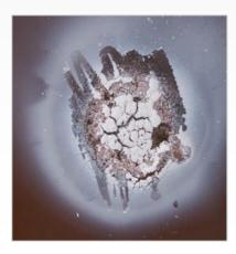
> 1,000 °C flame on a 1 mm silicone coated steel plate
