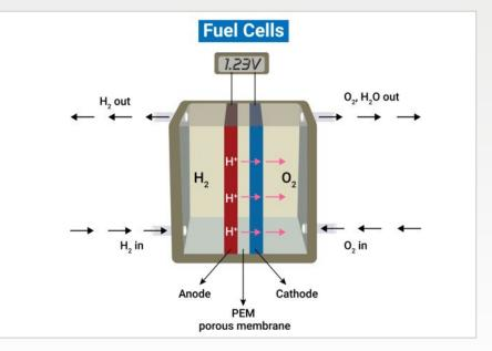
The most important type of fuel cell for many applications today is the proton exchange membrane fuel cell (PEMFC). Such a fuel cell usually uses hydrogen as fuel. This is generated either by steam reforming from methanol or methane and in the future from renevvable energy by electrolysis (green hydrogen).
