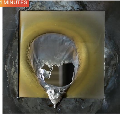
6061 T651 Aluminum (3mm) Breached in less than 4 minutes
