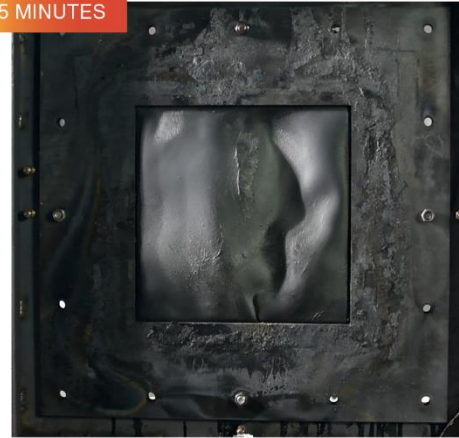
X-Protect RF0067K PA66 (3mm) Sustains direct flame for 15 minutes
