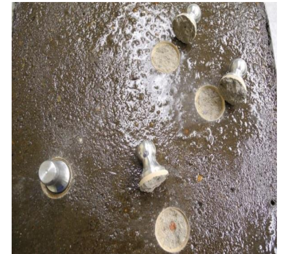
ASTM D7234 – bulk concrete failures
